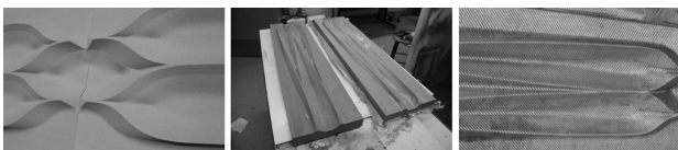
Figure 2. Renshape molds and fiberglass composite panel
